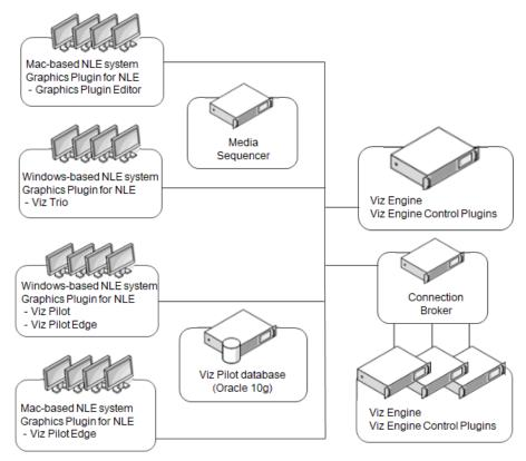
**Viz Engine** is a real-time graphics renderer, and at the core of the Vizrt graphics workflow. Viz Engine must handle multiple simultaneous requests. In Viz Engine, the multiplexing functionality is a built-in feature.
